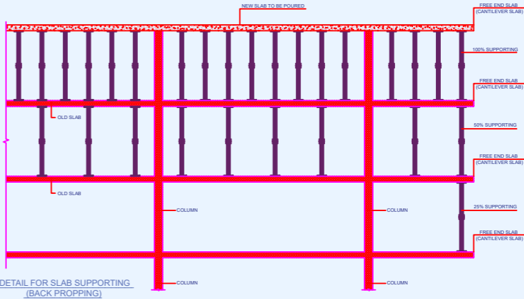
DETAIL FOR SLAB SUPPORTING (BACK PROPPING)
